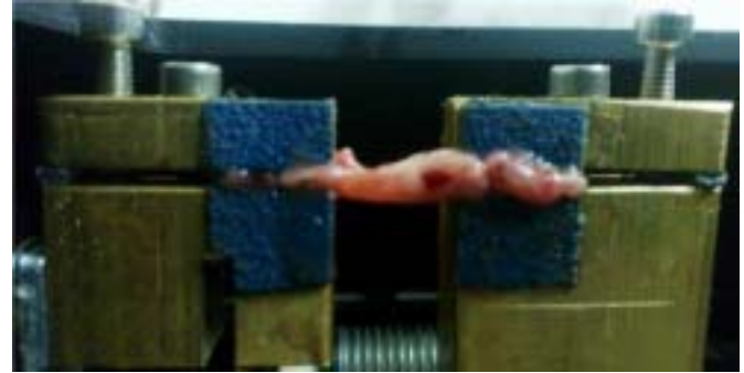
Figure 1: The tissue samples were placed at the ends of the transducer parallel to the uterine incision performed
